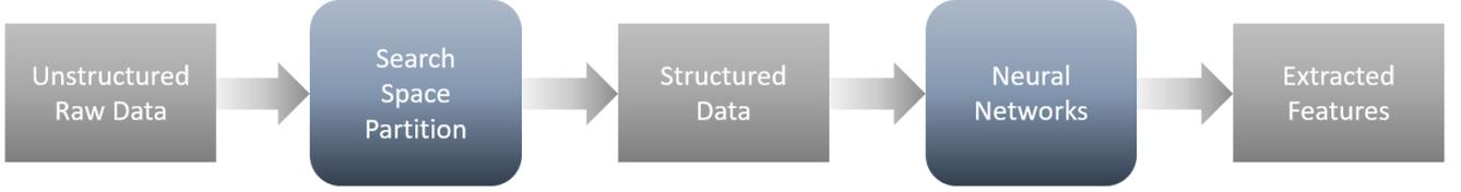
Fig. 4. Illustration of the data post-processing pipeline. Unstructured raw data descriptive of a solution population  $P_g^r$  at generation  $g$  and run  $r$  in the form of tuples  $(\mathbf{x}, f(\mathbf{x}))$  of candidate solutions and fitness values are converted by a search space partitioning method into a structured data format  $\mathbf{z}$ , which subsequently can be fed to an adequate neural network architecture for feature extraction.
